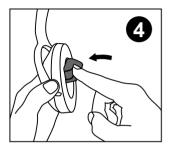
Firmly insert the new foam into the cup
