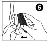
Align the ear pad with the cup and clip it into the cup
